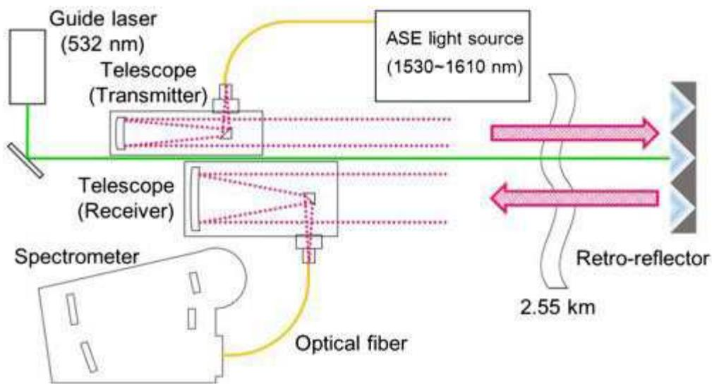
Figure 4: Example of an open path measurement system in which transmitter and receiver are in the one package and the measurement path is traversed twice (From Saito et al (2015))
