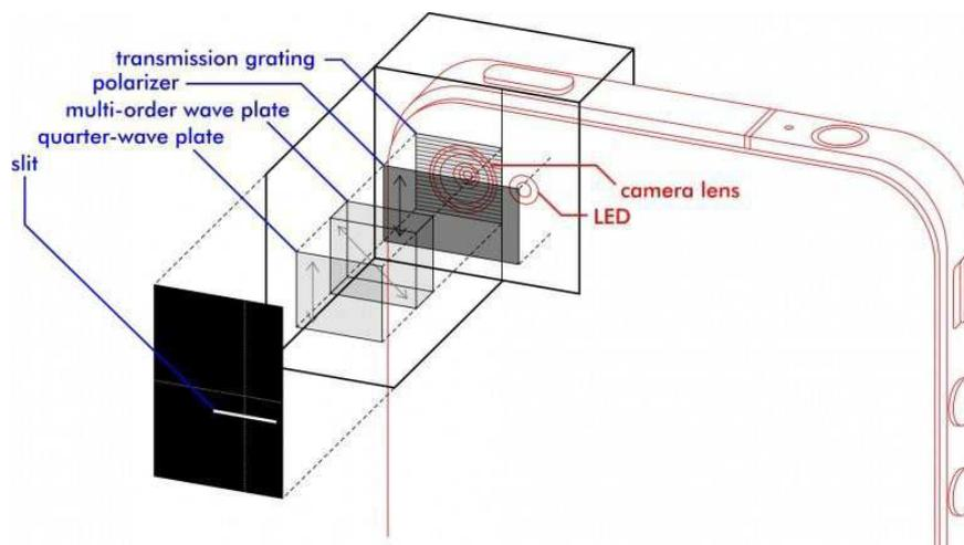
Fig 1: Reproduced from <http://ispex.nl/en/techniek/> showing the iSpex attachment to a smart phone
