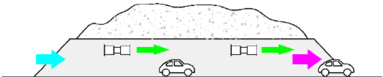
Figure 1: Longitudinal ventilation with jet fans
