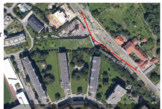
Figure 20: East portal with air quality monitoring paths, Nordspange Tunnel Graz, Austria, Source: Google Maps
